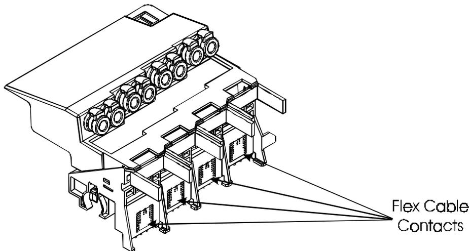
**Figure 3-3. Flex Cable Contacts.**
