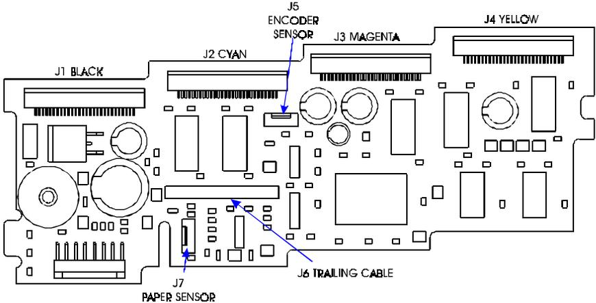
Figure 3-5. Carriage Connection Locations.
