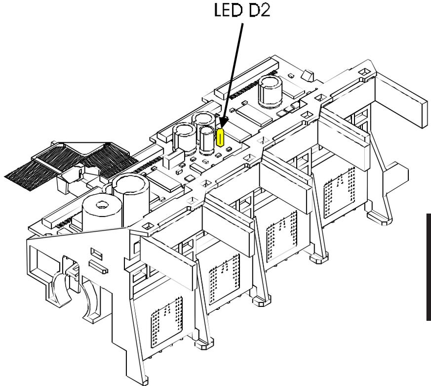
**Figure 4-1. Carriage Board LED D2 Location.**
