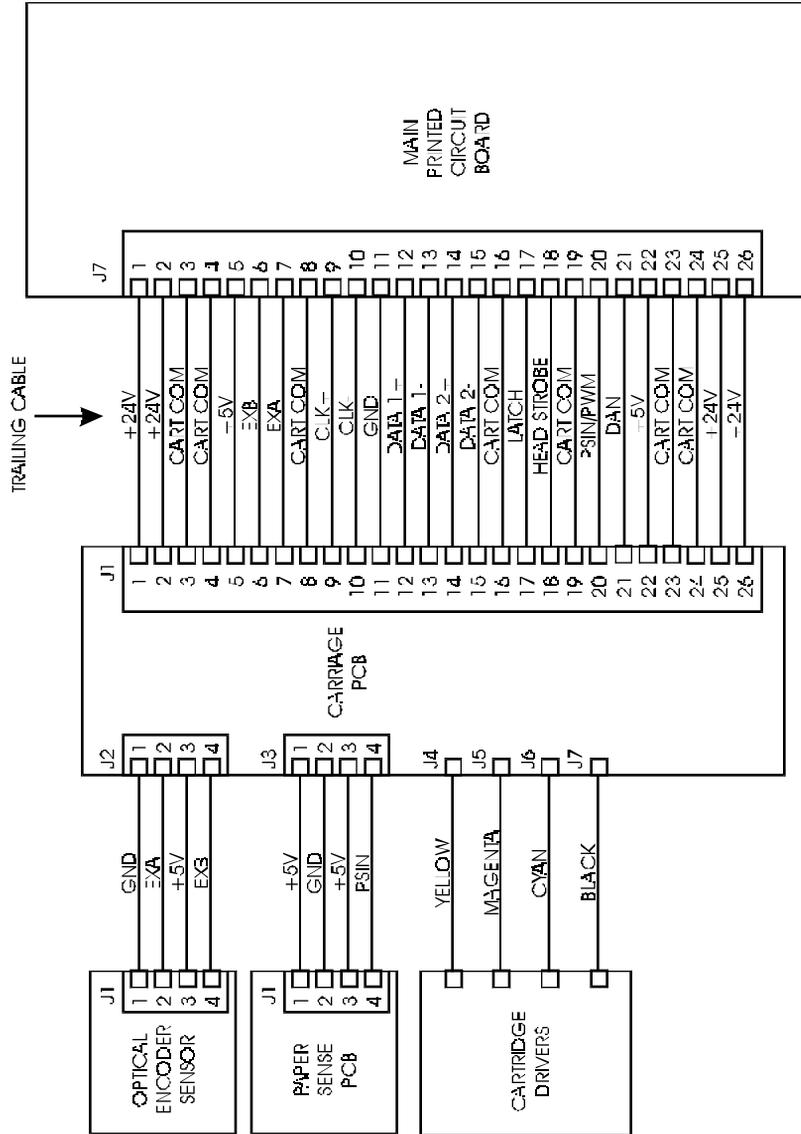
**Figure 3-31. Carriage PCB Connections Diagram.**
