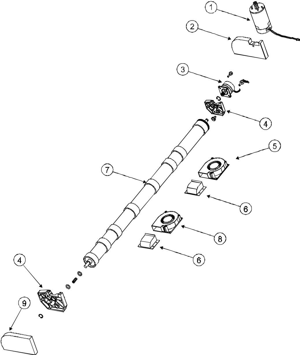
Figure 6-4. Inner Platen Parts Breakdown.
