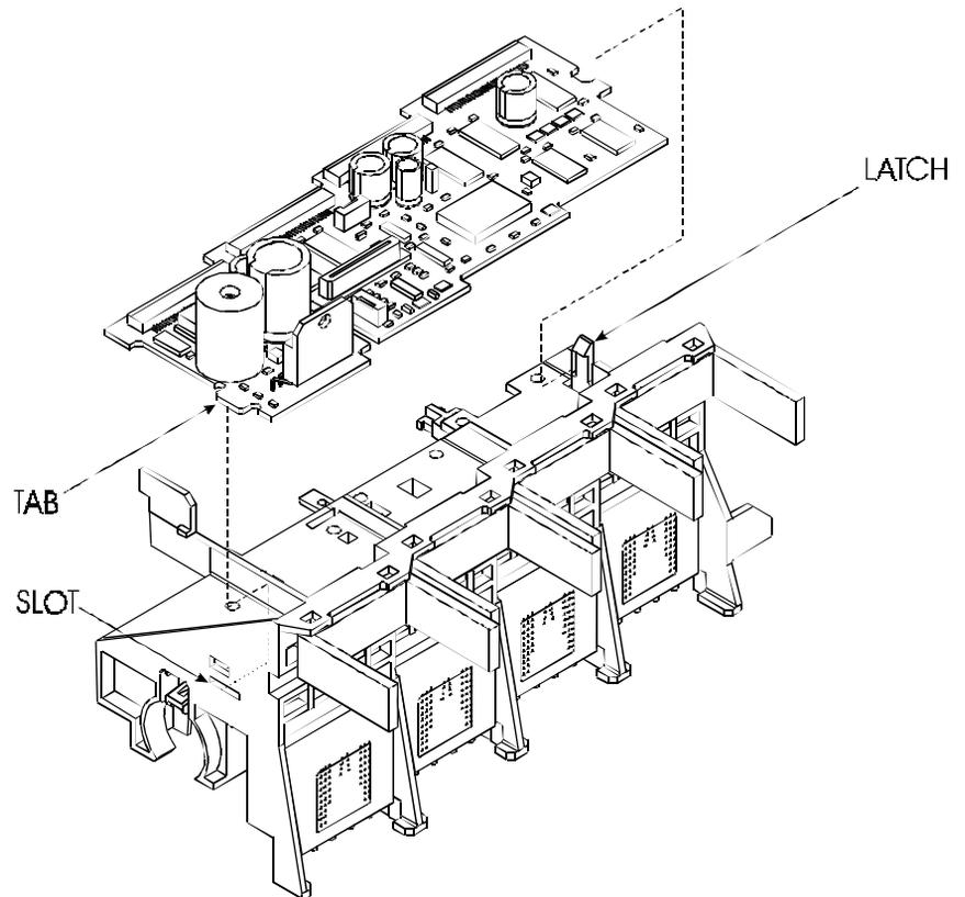
**Figure 5-15. Carriage PCB Removal/Installation.**
