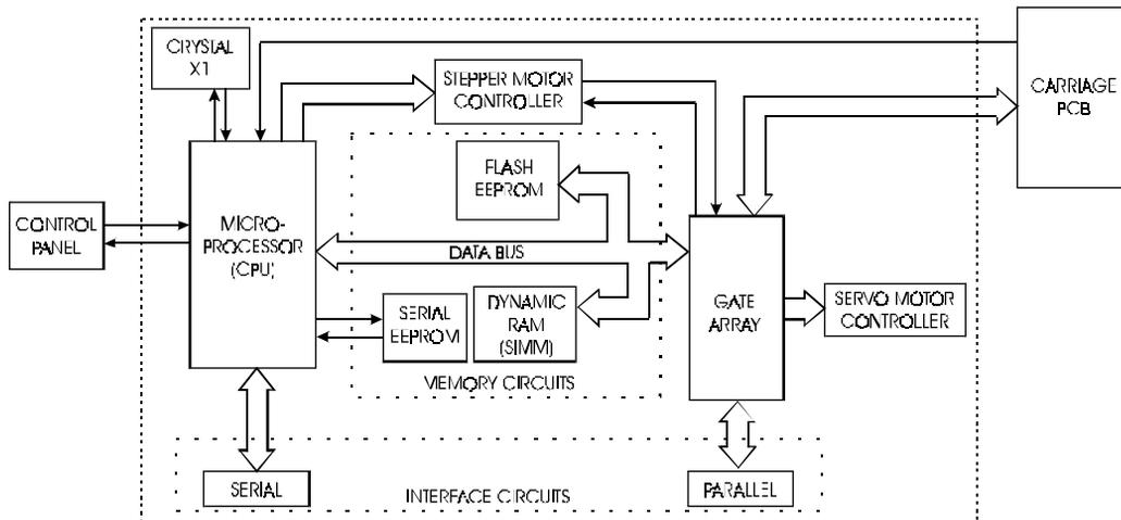
**Figure 2-5. Main Printed Circuit Board.**
