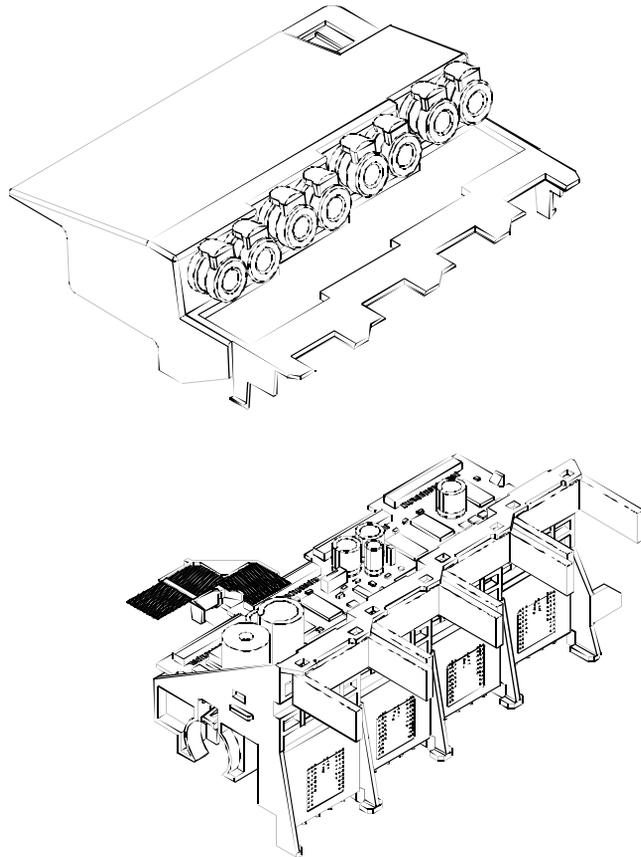
**Figure 5-10. Electronics Cover Removal.**
