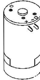
**Figure 3-9. Power Feed and Take-Up Motor.**
