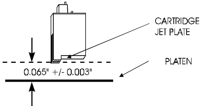
**Figure 3-14. Carriage Head Height Tolerance.**
