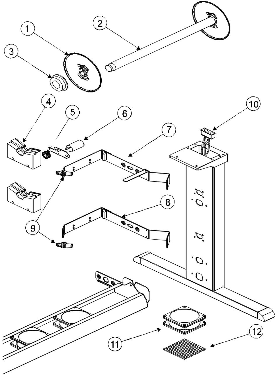
Figure 6-6. Power Feed and Take-Up Parts Breakdown.
