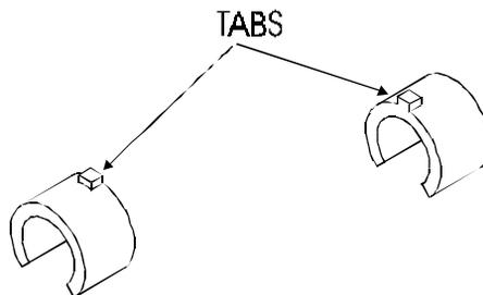
**Figure 5-19. Carriage Bushing Installation.**
