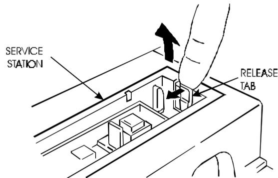
**Figure 5-20. Service Station Removal.**
