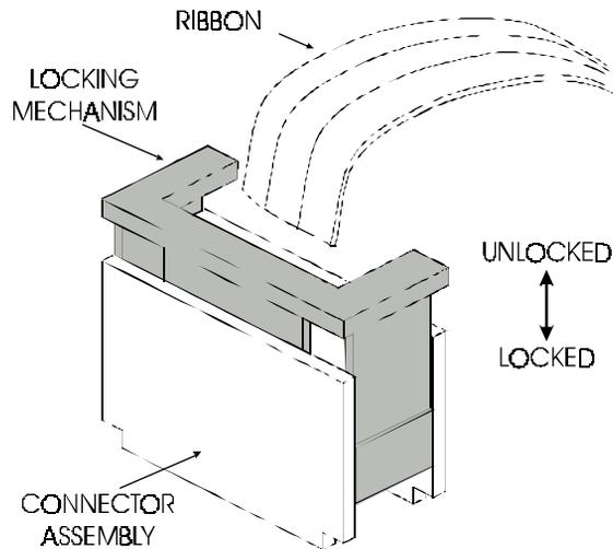
**Figure 3-6. Ribbon Connector Locking Mechanism.**
