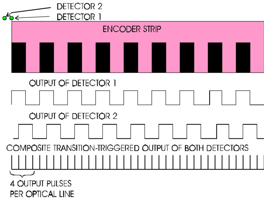
**Figure 2-9. Quadrature Signal Generation.**
