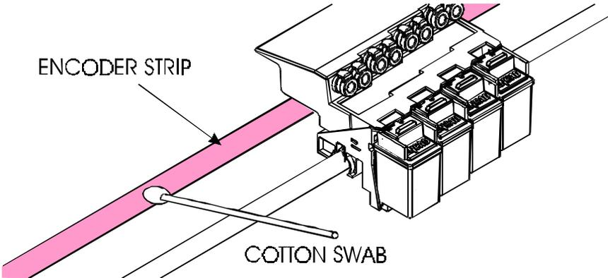
Figure 3-1. Encoder Strip Cleaning.
