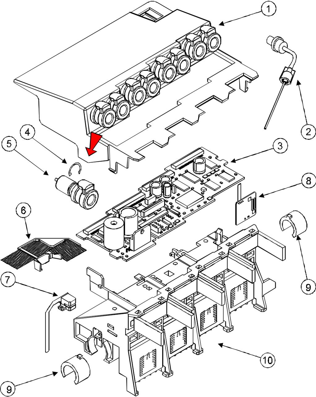
Figure 6-5. Carriage Assembly Parts Breakdown.
